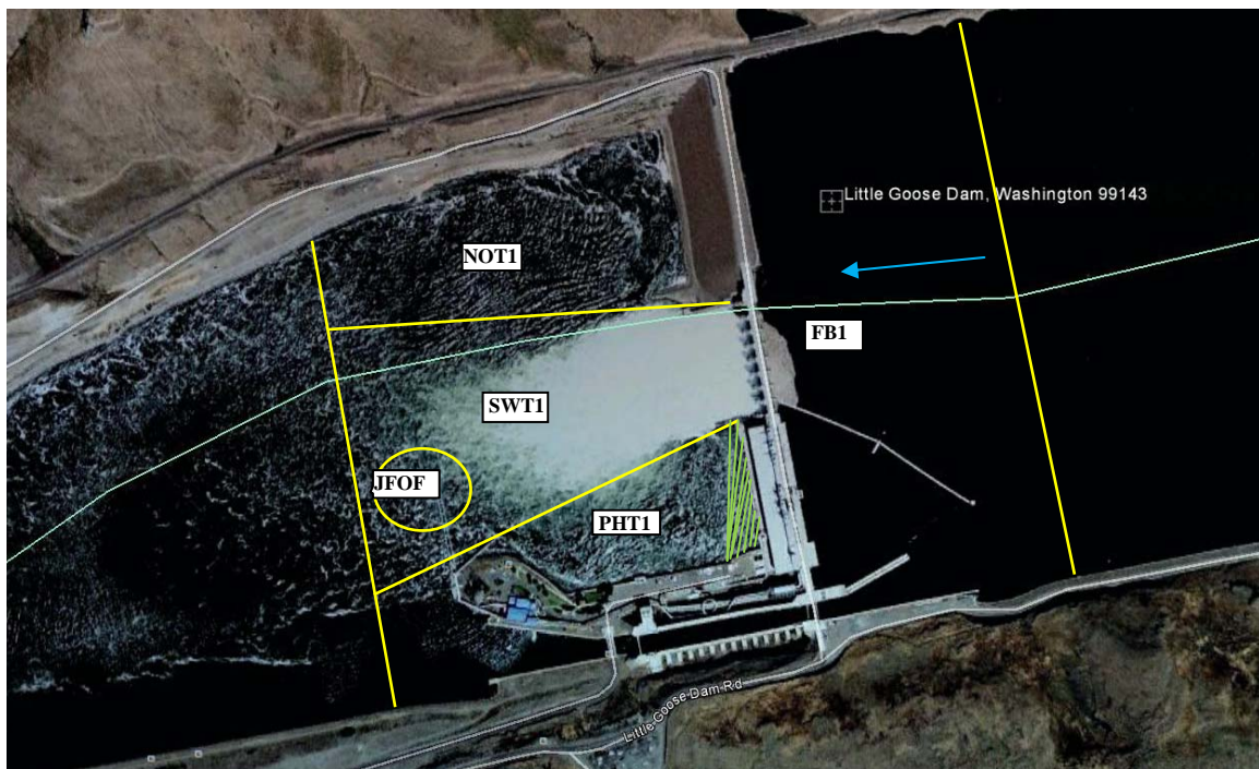
Figure 29. Zone map used at Little Goose Dam in 2013. Yellow lines demarcate zones, green lines represent the deterrent lines downstream of the powerhouse (not exact number), and the blue arrow indicates flow direction.
