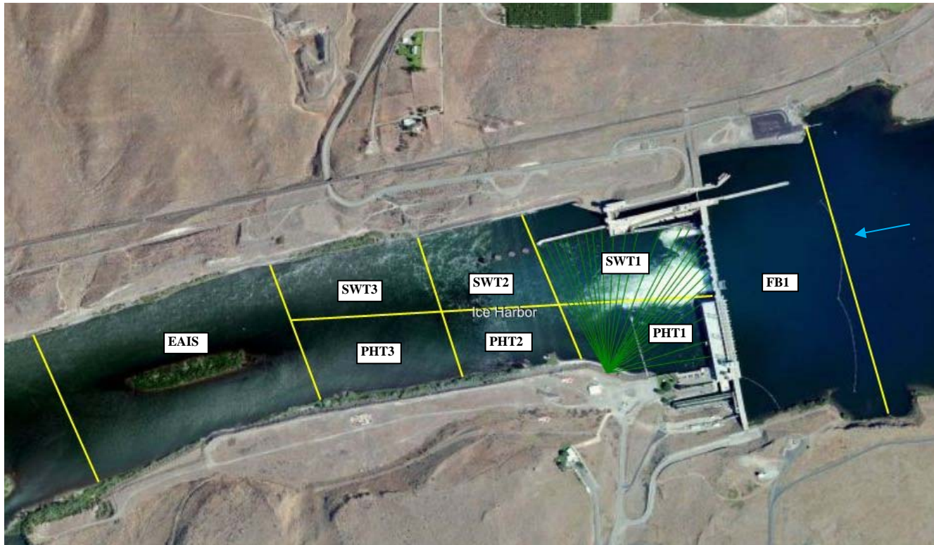
Figure 21. Zone map used at Ice Harbor Dam in 2013. Yellow lines demarcate zones, green lines represent the avian deterrent lines (not exact number), and the blue arrow indicates flow direction. Eagle Island Zone is approx 1.1 km downstream of the dam.
