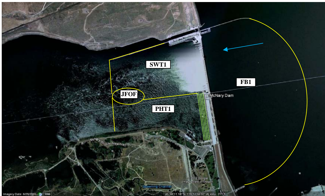
Figure 17. Zone map used at McNary Dam in 2013. Yellow lines demarcate zones, green lines represent the avian deterrent lines downstream of the powerhouse (not exact number), and the blue arrow indicates flow direction.
